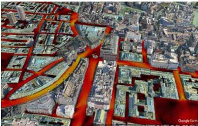
Fig. 4. Magnitude of time-averaged wind speed at ground level (1.5m) in the Piccadilly Circus area of London. West-East mesoscale wind direction.
