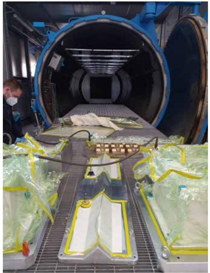
Fig 3. Available autoclave used for curing composite parts and prototypes.
