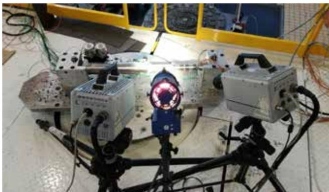
Fig. 1. Test setup with the actuator and the cameras positioned above the vibrating pot.
