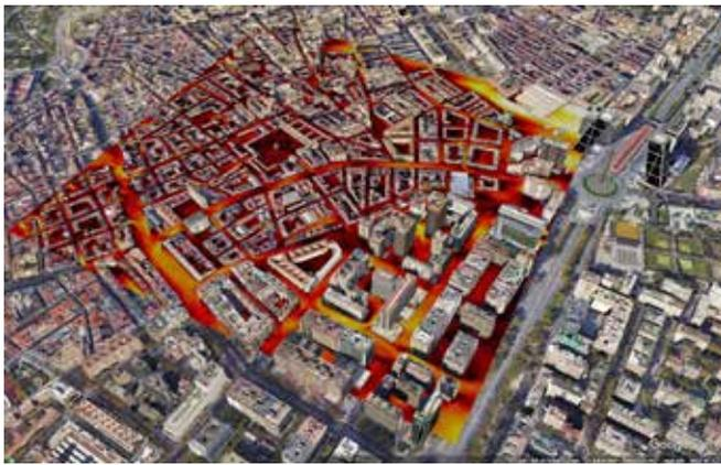
Fig. 3. Magnitude of time-averaged wind speed at ground level (1.5m) at Plaza Castilla in Madrid (Kio Towers on the right side of image). West-East mesoscale wind direction.
