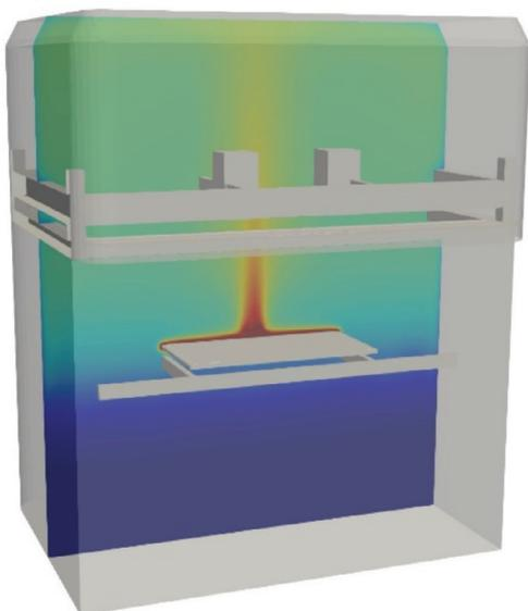
Figure 5: CFD model of 3D Printing Machine with temperature distribution.
