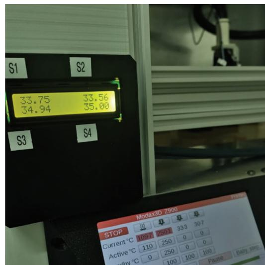
Figure 6: Experimental temperature measurement in 3d printer.
