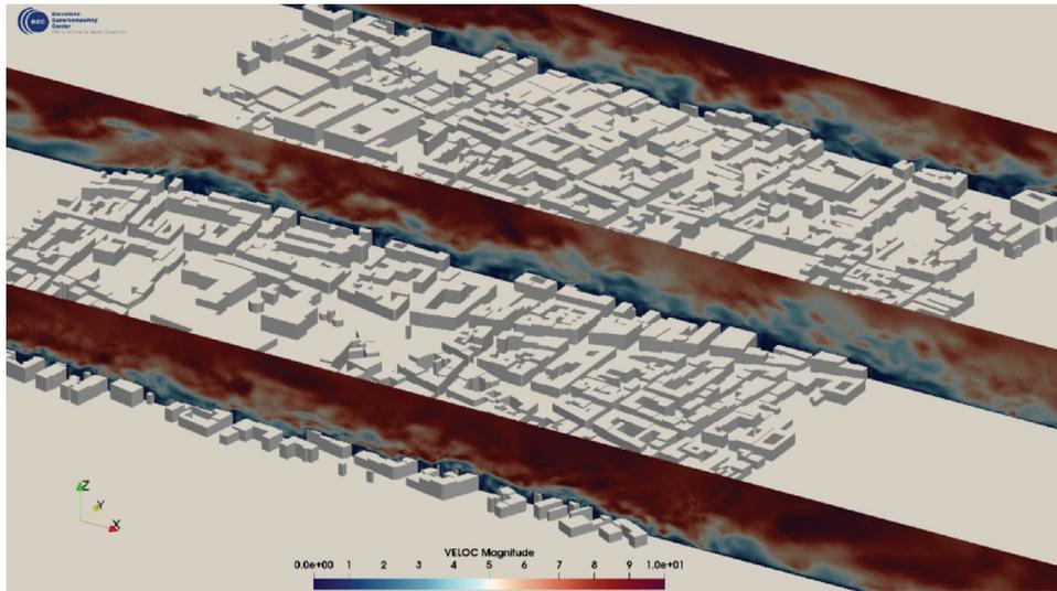
Figure 3: CFD simulation of a city geometry.
