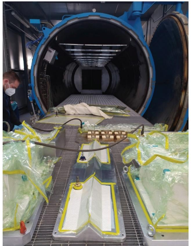
Figure 2: Autoclave for big composite parts.
